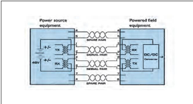
Power supply via data cables; Supply via the centre points of the isolating transformer:
