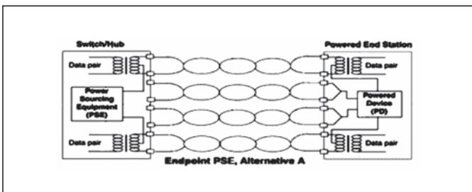
Power supply via free conductor pairs; Positive and negative voltage sides are transmitted via two conductor pairs
