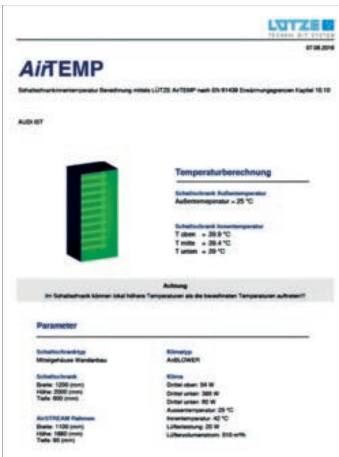
Figure 5: Thermal detail analyses with the LÜTZE AirTEMP software: The air-conditioning unit was not needed.
